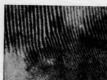
Fig. 3. Moiré pattern on tilt boundary. \times 100,000 .
